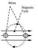
Maximum Voltage Wires cut across flux Minimum Voltage Wires move parallel with flux
