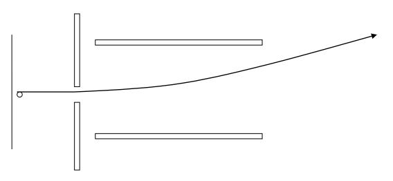
16a) If this were not done in a vacuum the accelerating electron would collide with the air gas molecules in the air and the electrons would be deflected or would be lost via ionisation with the molecules.
